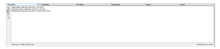
It takes about 196 ms (~196000 us). So that means to go from off to on and back to off again it will take twice this long or about 4 tenths of a second. This is how I knew that the LED was blinking about 2 1/2 times per second.
